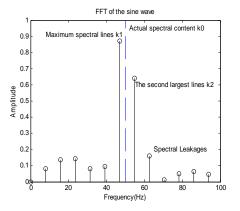
Figure 2. Frequency Spectrum of Asynchronous Sampling Signal
