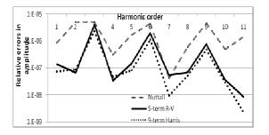
Figure 5. Comparisons of Relative Errors of Harmonic Amplitude
