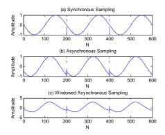
Figure 1. Asynchronous and Synchronous Sampling of the Same Signal
