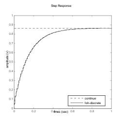
Figure 6. Step response of discrete system with FOH method
