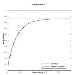
Figure 7. Step response of discrete system with impulse-invariant method
