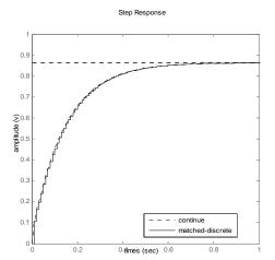
Figure 9. Step response of discrete system with matched method
