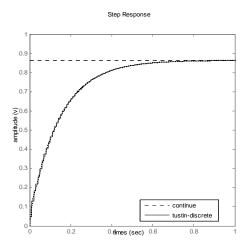
Figure 8. Step response of discrete system with Tustin method
